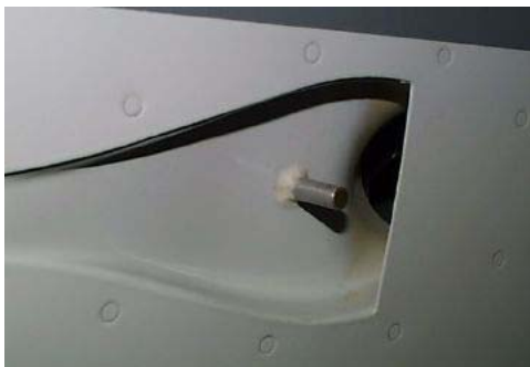
Possible temperature probe installation location
