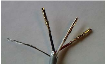
Picture 1: Properly crimped pins.
